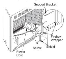
Figure 16 - Installing Shield to Support Bracket
